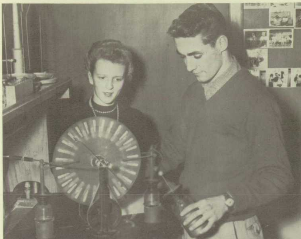
Jo Ann Jahn and Mike Witte are storing electricity in a Leyden jar by using the static electricity machine.
