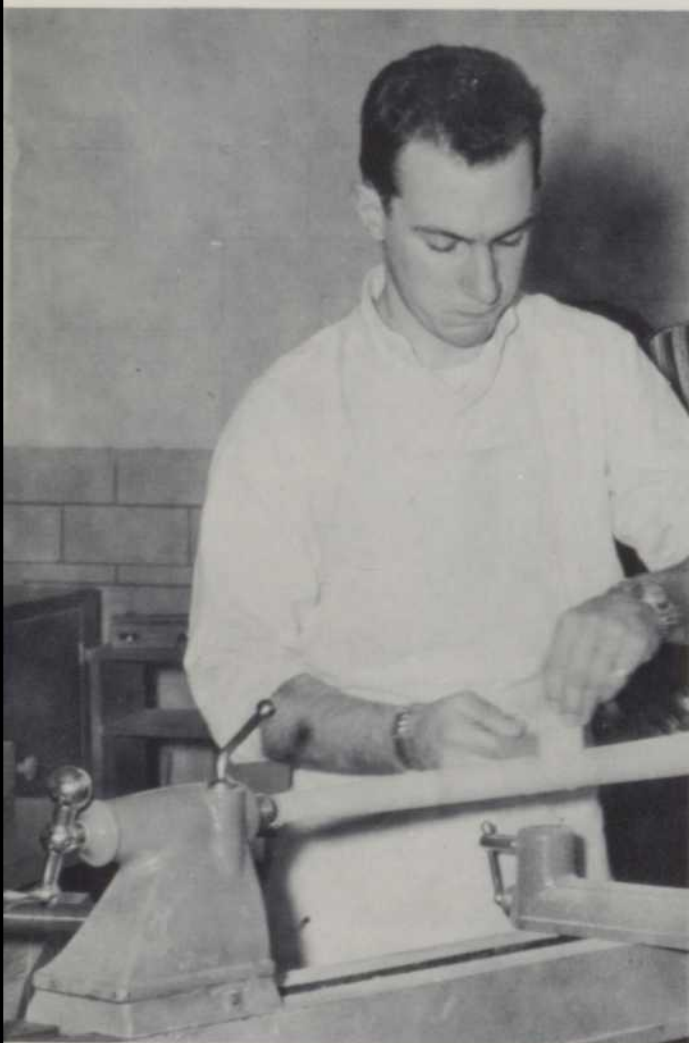
Using the power lathe in the woodworking shop, senior Dave Buehler turns out a part for a project which is required of all shop students.
