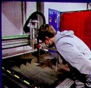
Brandon Schnell working on the Plasma Cutter using metal to cut out trees and logos for a project.
