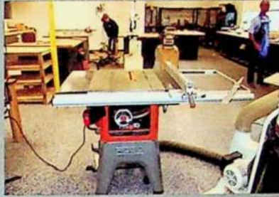
The tablesaw is for cutting longer pieces of wood.
