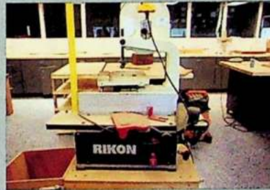
This is a bench top jointer, it gives the wood a good edge.
