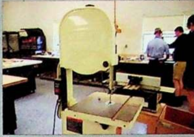
The vertical saw is for cutting small corners and difficult pieces.
